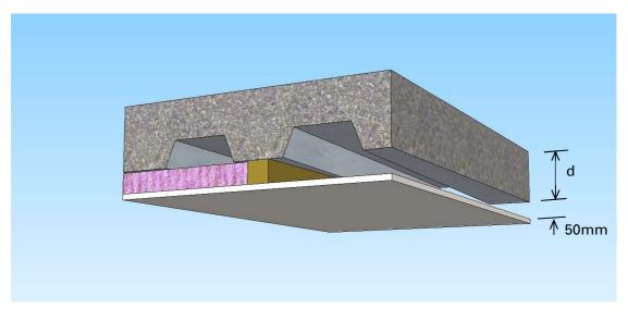
Figure 1. ComFlor 60 showing Battened Ceiling
