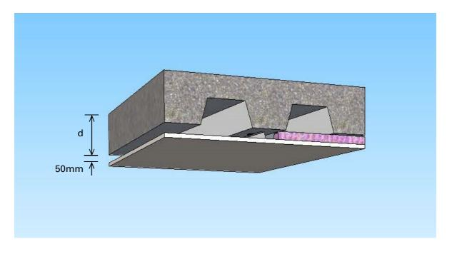
Figure 2. ComFlor 80 showing Ceiling on Resilient Clip
