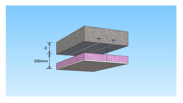
Figure 4. ComFlor SR showing Suspended Ceiling
