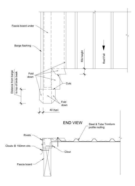
Rib Profile Barge Eaves Detail Plan View
