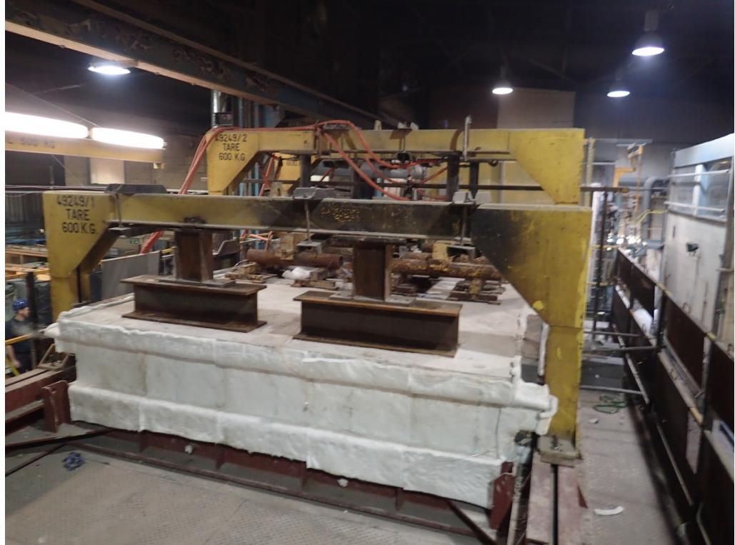
The unexposed face of the test specimen after a test duration of 30 minutes
