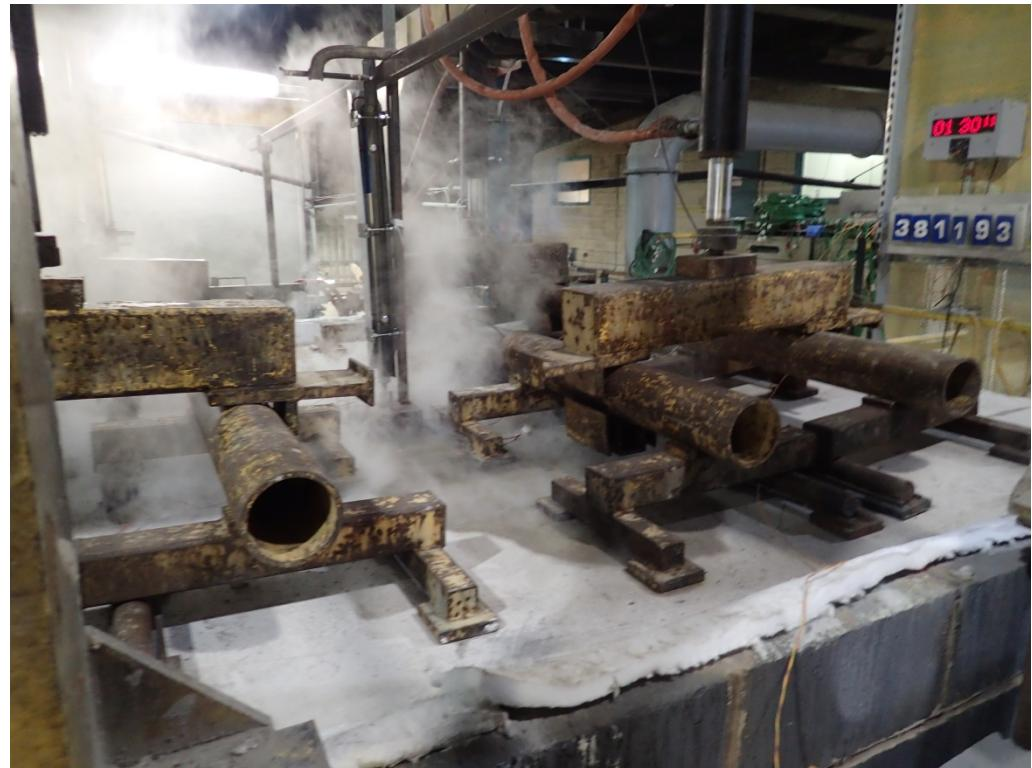
The unexposed face of the test specimen after a test duration of 120 minutes
