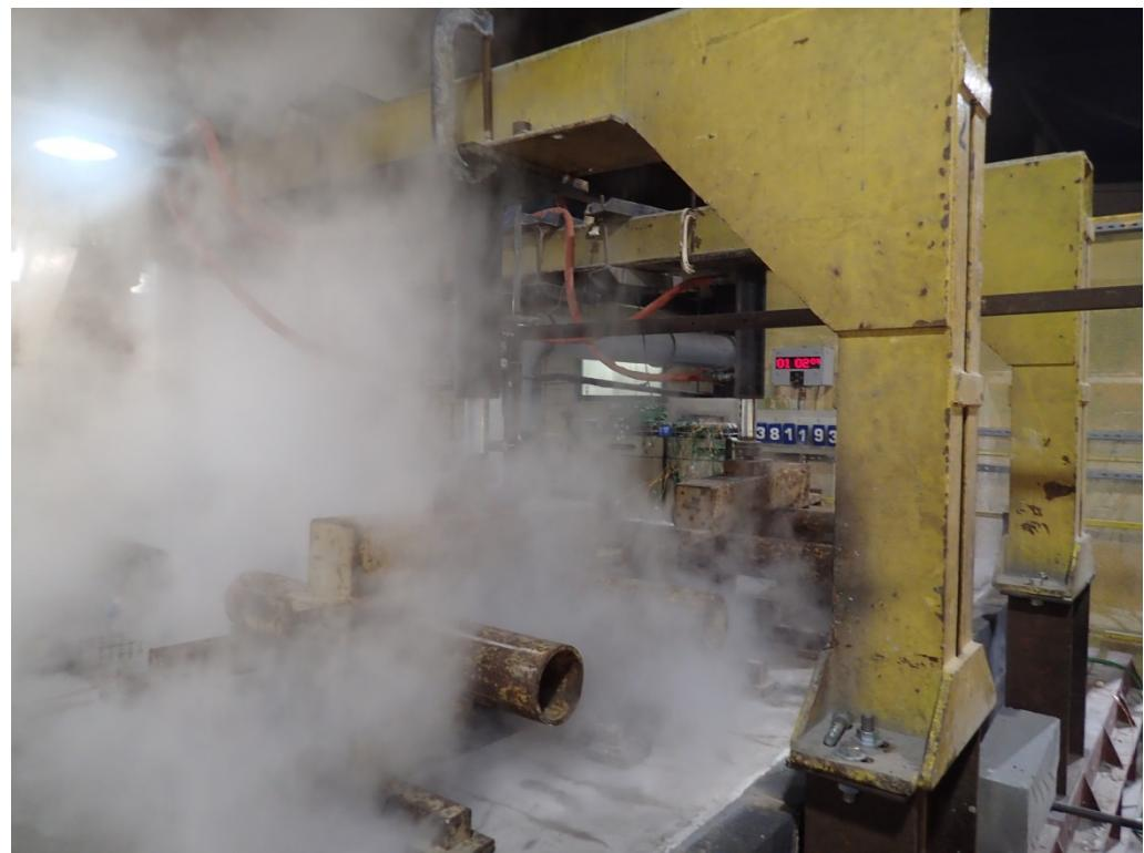
The unexposed face of the test specimen after a test duration of 90 minutes
