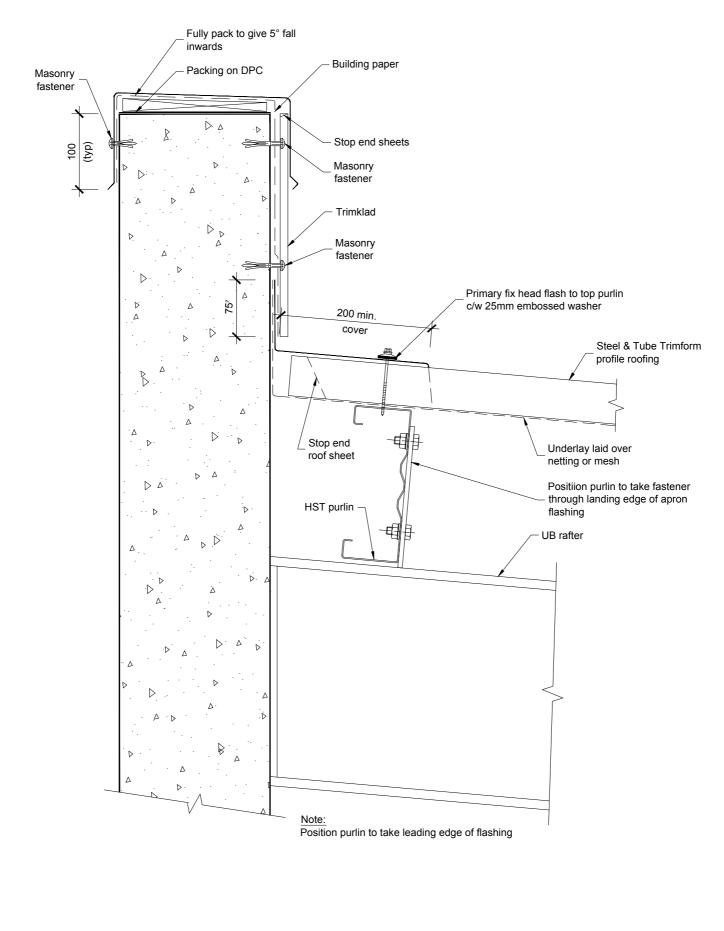
Lined Parapet Head Flashing **Cross Section**
