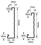
An attractive and economical advance over timber fascias, **Multiline Fascia** can be fitted with a range of spoutings for contemporary or traditional appearances.  Multiline Fascia uses a uniquely designed rafter bracket to prevent denting and damage in metal fascias due to differential movement of trusses and rafters.
