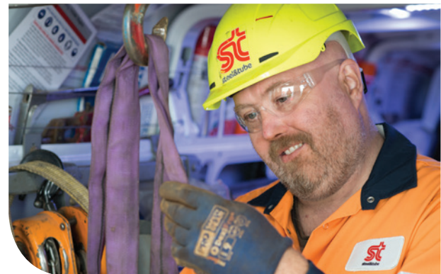
Technician visually inspecting synthetic sling.
