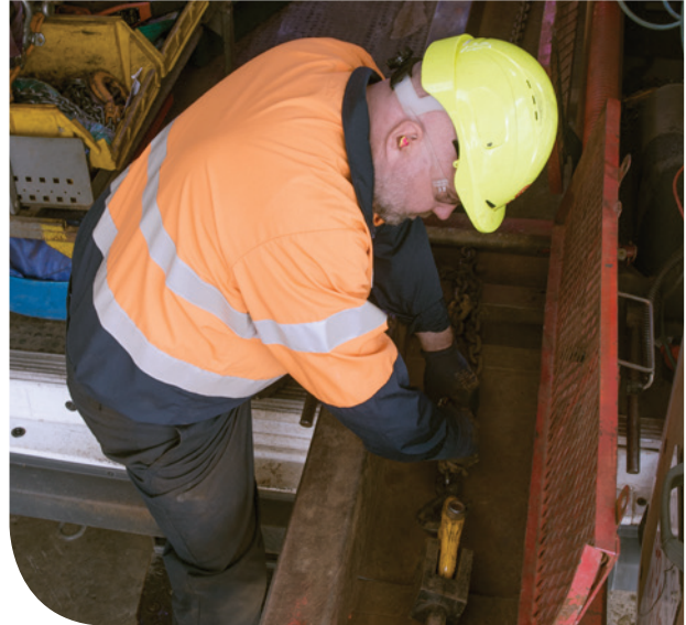
Technician proof loading chain on-site in mobile testing van.
