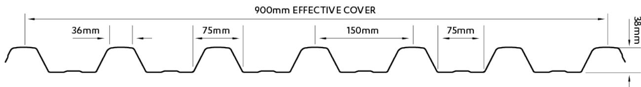
ST900® is a medium rib profile. Developed for the commercial/industrial roofing and cladding markets, it is equally at home in residential settings where a bolder look is desired.
