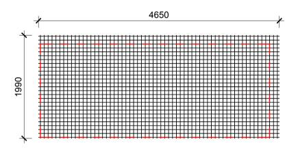
Type Name:335L Width:1990.0 mm Length:4650.0 mm Pitch:75.0 mm Cover Width:1800.0 mm Cover Length:4425.0 mm Cover Area:7.97 m² Wire Size (Main):5.3 mm Wire Size (Edge):5.3 mm Ribbed:No
