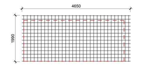
Type Name:663L Width:1990.0 mm Length:4650.0 mm Pitch:150.0 mm Cover Width:1750.0 mm Cover Length:4300.0 mm Cover Area:7.53 m<sup>2</sup> Wire Size (Main):6.3 mm Wire Size (Edge):6.3 mm Ribbed: Yes
