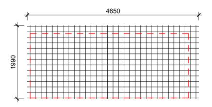
Type Name:668L Width:1990.0 mm Length:4650.0 mm Pitch:150.0 mm Cover Width:1750.0 mm Cover Length:4300.0 mm Cover Area:7.53 m² Wire Size (Main):4.0 mm Wire Size (Edge):4.0 mm Ribbed:Yes
