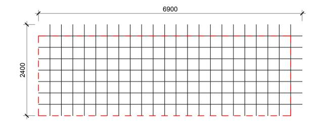
Type Name:212ST Width:2400.0 mm Length:6900.0 mm Pitch:300.0 mm Cover Width:2100.0 mm Cover Length:6600.0 mm Cover Area:13.86 m<sup>2</sup> Wire Size (Main):9.0 mm Wire Size (Edge):9.0 mm Ribbed: Yes
