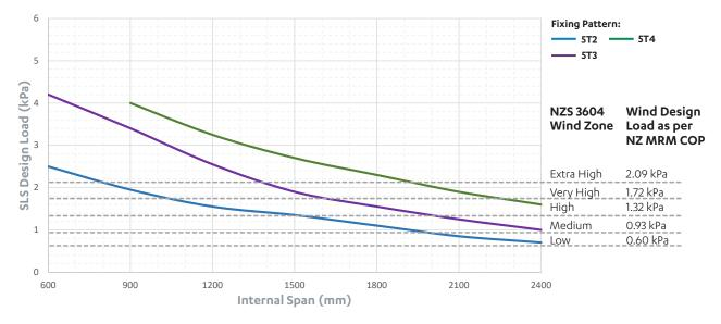
H36 0.90 BMT ALUMINIUM PLUMBDEK® SERVICEABILITY LIMIT STATE (SLS) WIND LOAD GRAPH
