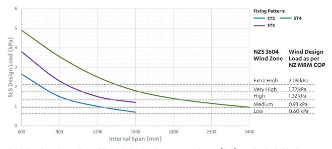
G550 0.55 BMT STEEL PLUMBDEK® SERVICEABILITY LIMIT STATE (SLS) WIND LOAD GRAPH
