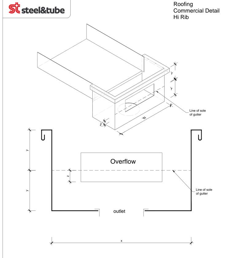
Dimension y equal to Depth of gutter at outflow
