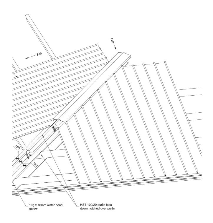
Netting and underlay omitted for clarity Stopend top edge of sheet
