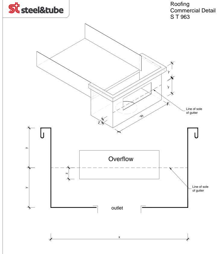
Dimension y equal to Depth of gutter at outflow
