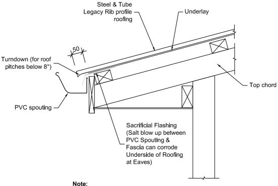
Eaves flashing required for durability in severe marine conditions where PVC or other low front spouting is used.
