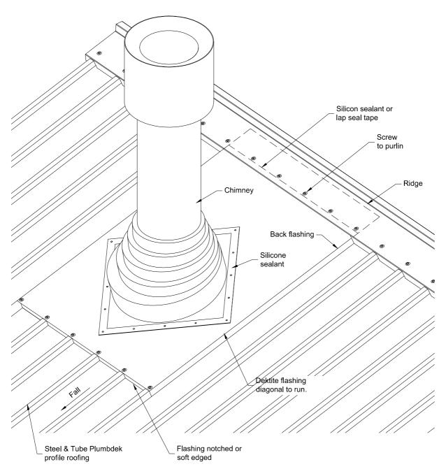
Note: Soft edged flashings to be colour matched prior to installation.
